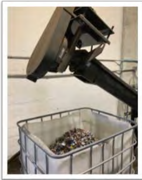
Aluminum is separated from coffee grounds via food-grade turbo separator
